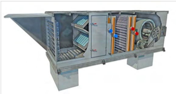
Figure 5. Rooftop air handling unit with economizer provisions
